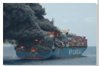
FIREWORKS in 7 containers reportedly contributed to damages aboard the *Hyundai Fortune in March 2006* while an investigation revealed an explosion below deck, near the ship's engine compartment, which actually caused the fire. Reportedly, some 60-90 containers tumbled into the ocean.
