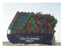
WAVES can do a lot of damage to cargo, and the vessel itself. Above is the brand new ship Ital Florida, on its maiden voyage from Hong Kong in June 2007. En route the ship was pounded with wave heights between 22' - 32' feet that caused the "stack attack" shown above. The ship itself is 783 ft long, and weighs 36,483 tons gross.
